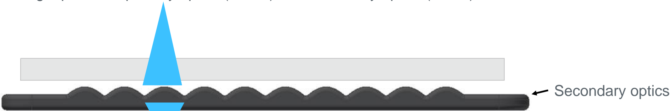
Light path with primary optics (above) and secondary optics (below).
