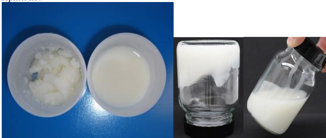
Figure 1: Example same 100% UV formulation, at 12% silica loading, hyper-branch co-polymer dispersant on right has superior flow
