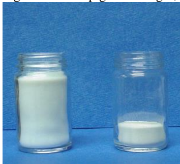
Figure 8: Same pigment weight, different bulk densities of Pyroengenic Fumed Silica (left) vs. MMT (right)
