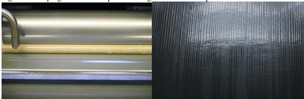
Figure 3: “Roping marks” from poor leveling on 100% UV topcoat
