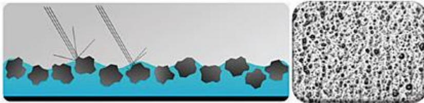
Picture 6. Matting through particle based light scattering.
