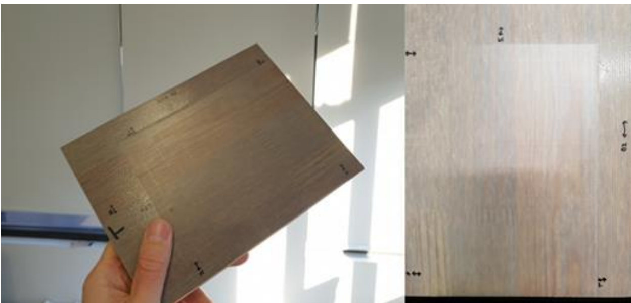
Picture 16. A glossy wood coating made matt (gloss 10) with the MicroTau DCM technology, including the developing step.
