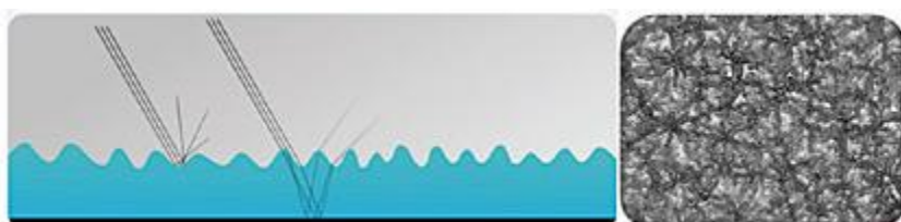
Picture 9. Matting through Excimer induced surface wrinkling.
