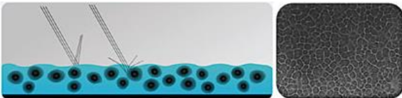
Picture 8. Matting through internal reflection, utilizing waxes
