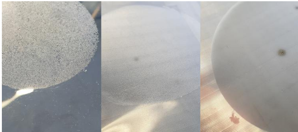
(a) Condensation forming, from left-to-right, on an untreated surface; a crosshatch microstructured surface; and a finer crosshatch microstructured surface.
