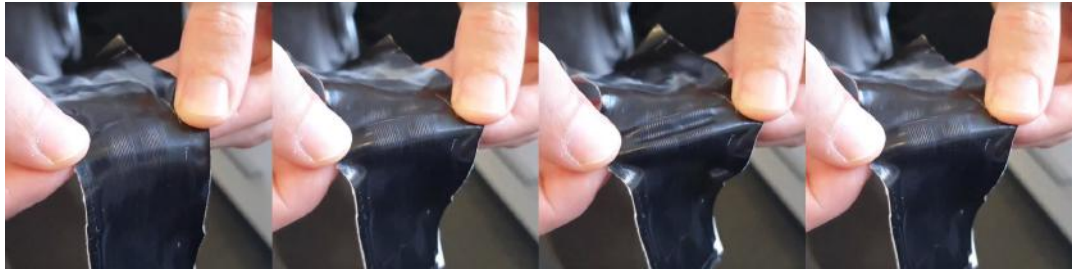
Figure 10. Riblets fabricated on a textile substrate. Frames from a video demonstrating ability to be stretched and return to original form.
