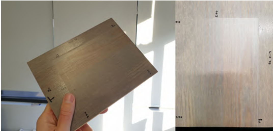
Figure 7. Matte properties imparted in a glossy wood UV curable coating with the DCM process.
