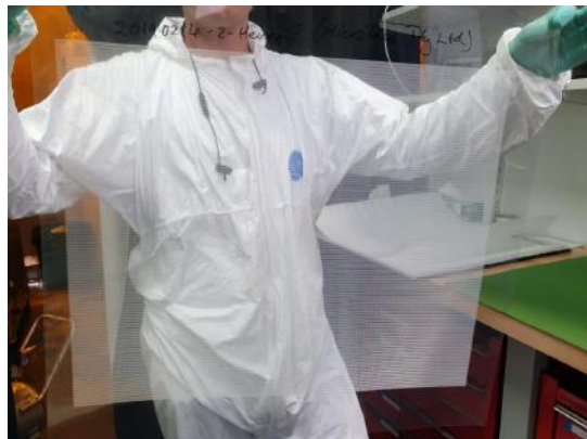
Figure 9. Example of 3D riblet film produced with the DCM film-printing process. MicroTau is building a pilot film printing capability to fulfil custom microstructure films orders.
