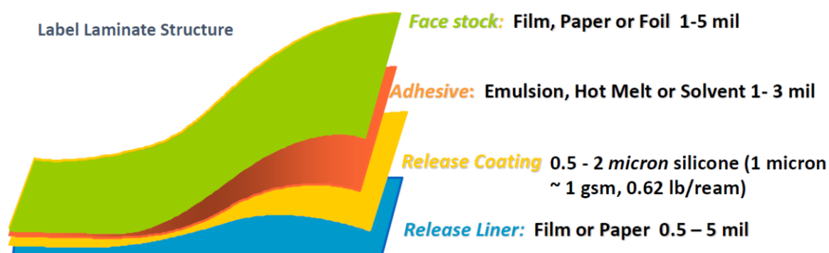
Figure 1: Label laminate construction
