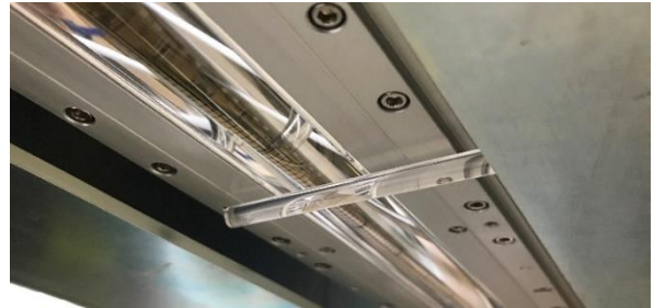
Figure 6. A picture of ICAD in action, measuring an LED array.
