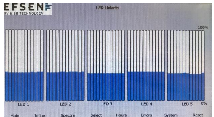
Figure 8. A measurement of 5 pcs AC8300-395 UV LED heads after “calibration” of heads.
