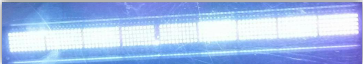
Picture 1. Close-up of 9 UV LED sections with one (no.4) being faulty (Courtesy of Excelitas/OmniCure)
