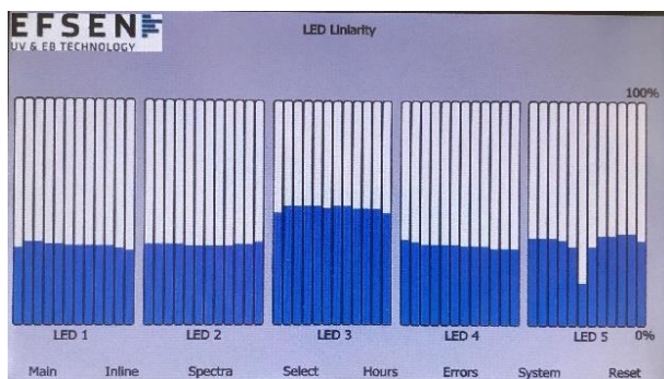
Fig 1 measurement of W-LED inline (5 heads)
