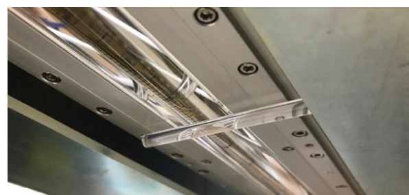
Picture 2. Close-up of ICAD® rod under UV LED
