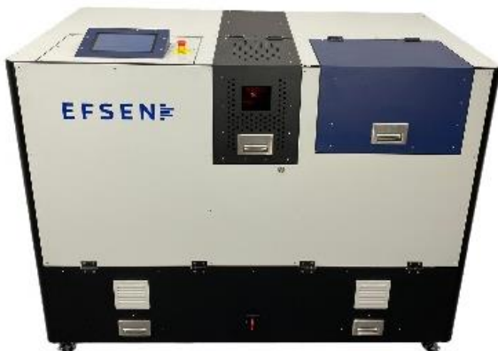
Picture 7-8. ICAD® Test Bench used for Hg-based lamp systems
