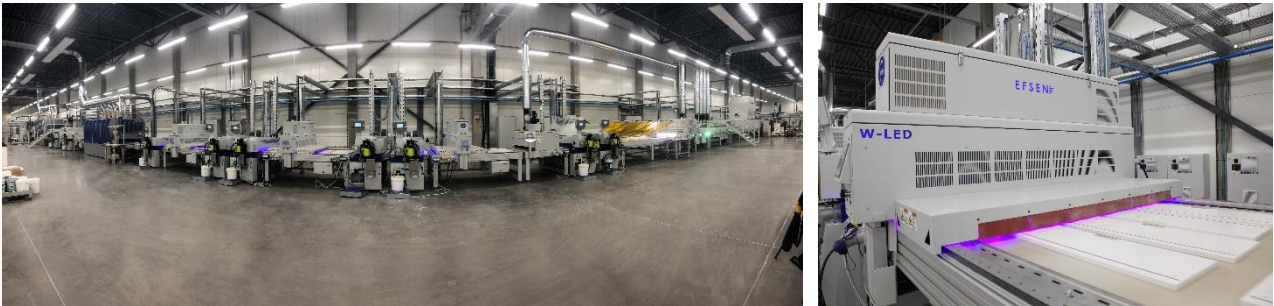
Picture 3-4. Furniture line with 7 W-LED with ICAD® and one stand-alone W-LED with ICAD®
