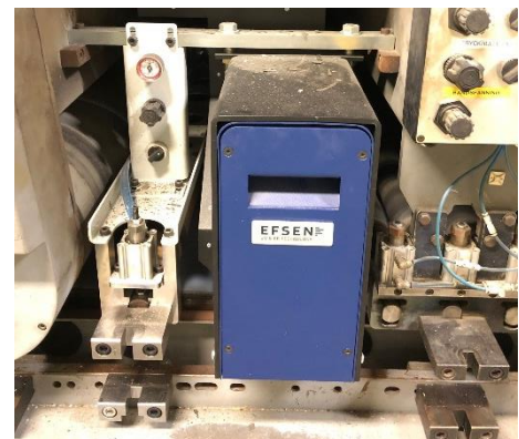
Picture 5. P-LED with ICAD® build into a curing oven with a foil running between LED and surface of product
