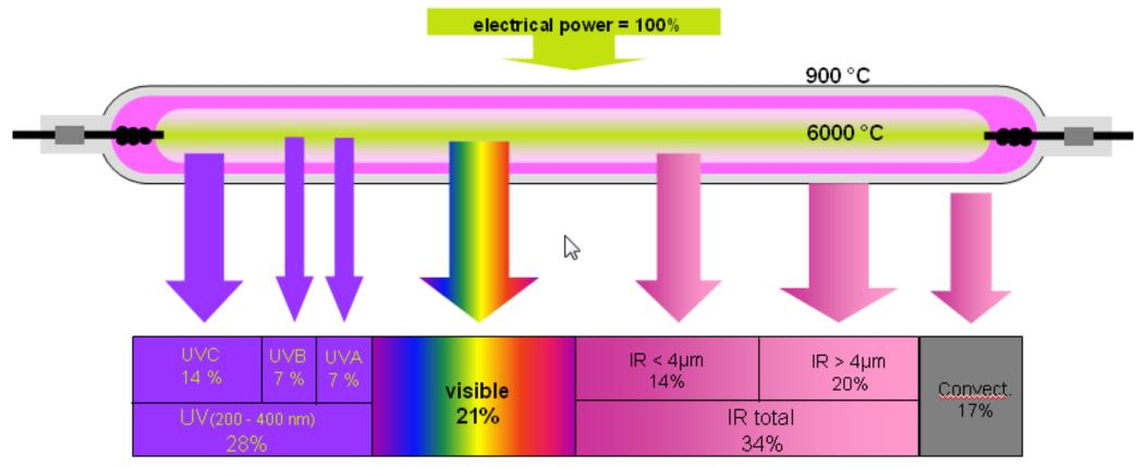
Typical characteristics for standard Hg lamp according to [Lambrecht 1999]
