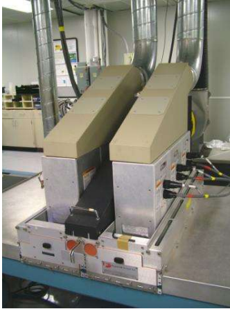
Photo 4.) UV Microwave (electrodeless) cure lamp
