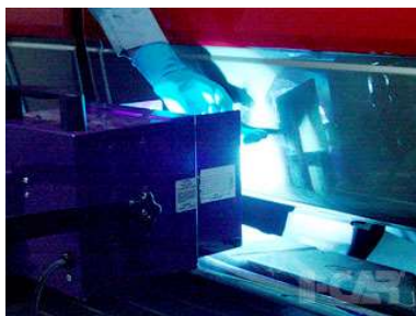
Photo 3.) UV A only light source used by the Automotive Refinish industry (Photo provided by I-CAR)
