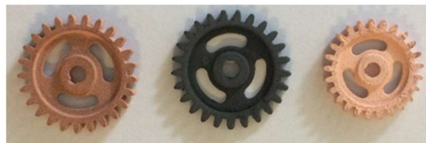
Figure 5. SLA copper structures Green copper part (Cu F1), debinded part and sintered part (left to right)
